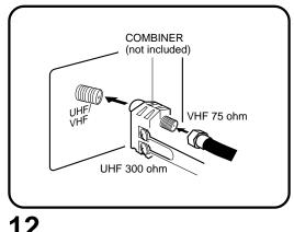
Connect the VHF 75 ohm cable and UHF 300 ohm twin-lead wire to the combiner. Attach the combiner to the antenna jack.
